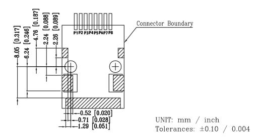
5-3. Recommended PWB Layout (Component Side View):
